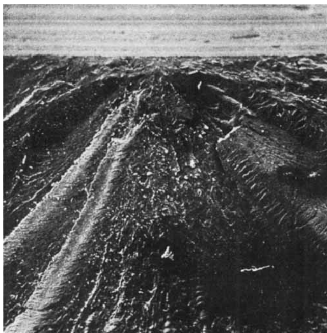
Fig. 26. Electron-scanning micrograph ( \times 55 ) of fracture surface of a notched Izod specimen of sample E, broken at -20^{\circ}\text{C} (see Fig. 24). White area is the notch surface.
